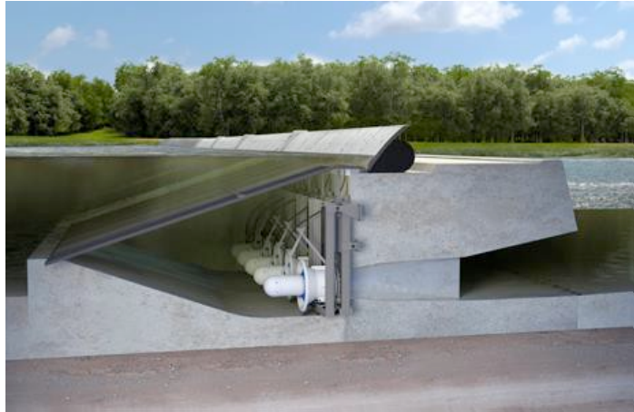
Fig. 5. The pictured structure is a compact turbine for low-head applications that can be integrated into existing weir systems or transfer structures to minimize civil construction. It has water-lubricated bearings and standardized frame sizes.
