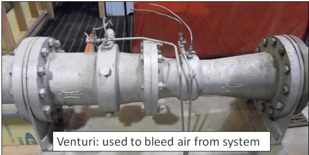
Figure E.5 Close-up of Venturi within Experimental Set-up
