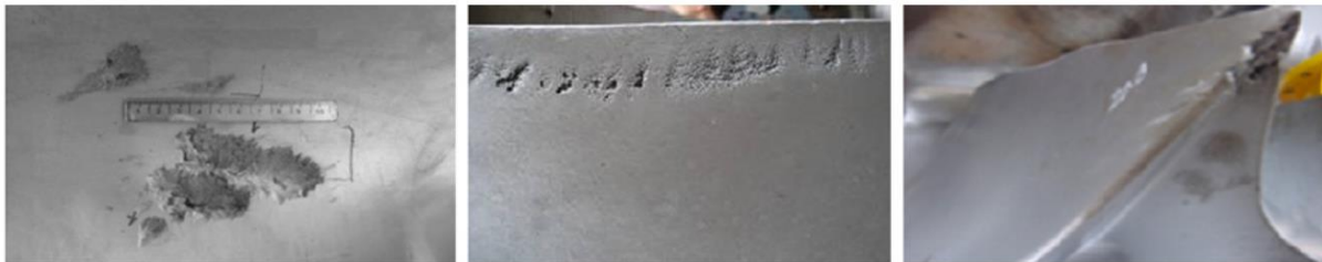
Figure 1.2: Cavitation erosion marks in a Pelton turbine 61
