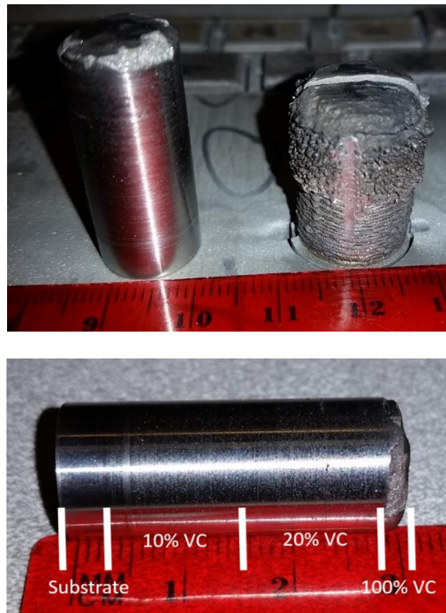
Figure 3.16: (Top) Image of machined cylinder and as built cylinder. (Bottom) Machined gradient cylinder.
